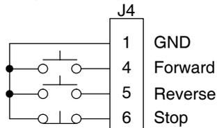
Note: Simultaneous closure of J4-4 and J4-5 will cause the motor to decel to stop if the motor is running. If the control is in a fault condition, simultaneous closure of these inputs will attempt a fault reset.
