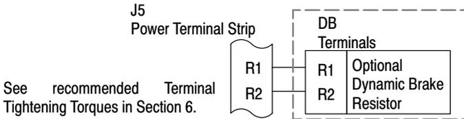
Note: Although not shown, metal conduit should be used to shield all power wires and motor leads.
